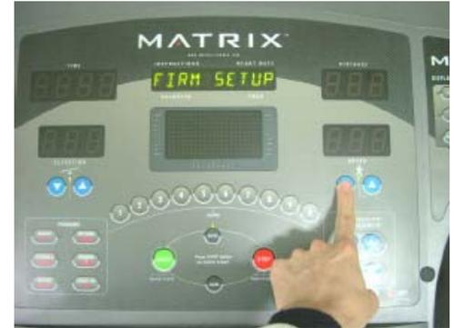
To enter Engineering Mode Continue to hold keys, and scroll to Firm Setup press Enter
